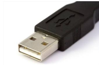
Rule of thumb: The USB end (see picture) goes into the computer, while the smaller end goes into the camera!
